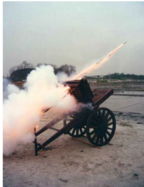
Rockets in Ancient Korea. Fig. 11 Flight test of small and medium Sin-Gi-Jeon at Daejeon Expo 93.
